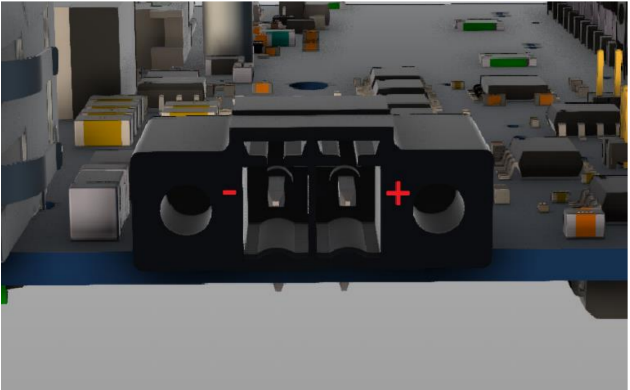
Figure 4: Power connector J3 polarity.
