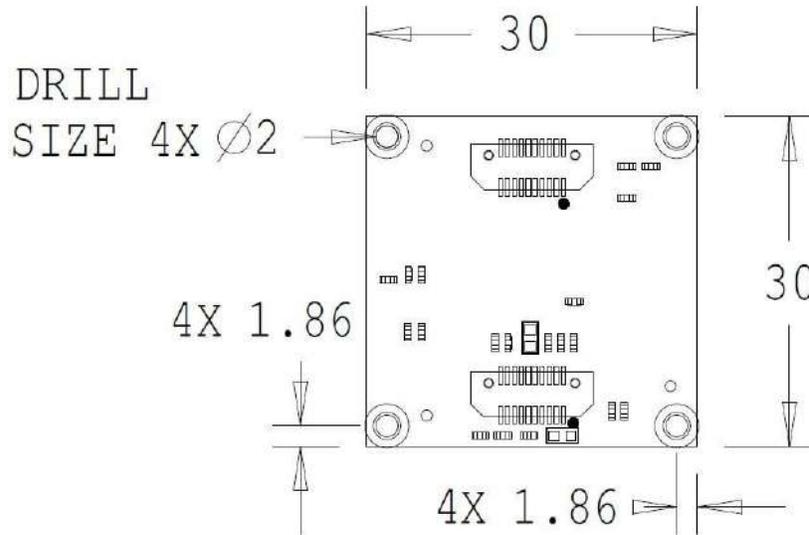
Figure 1: e-CAM50\_CUIMX8 Camera Adaptor Board Mechanical Dimensions
