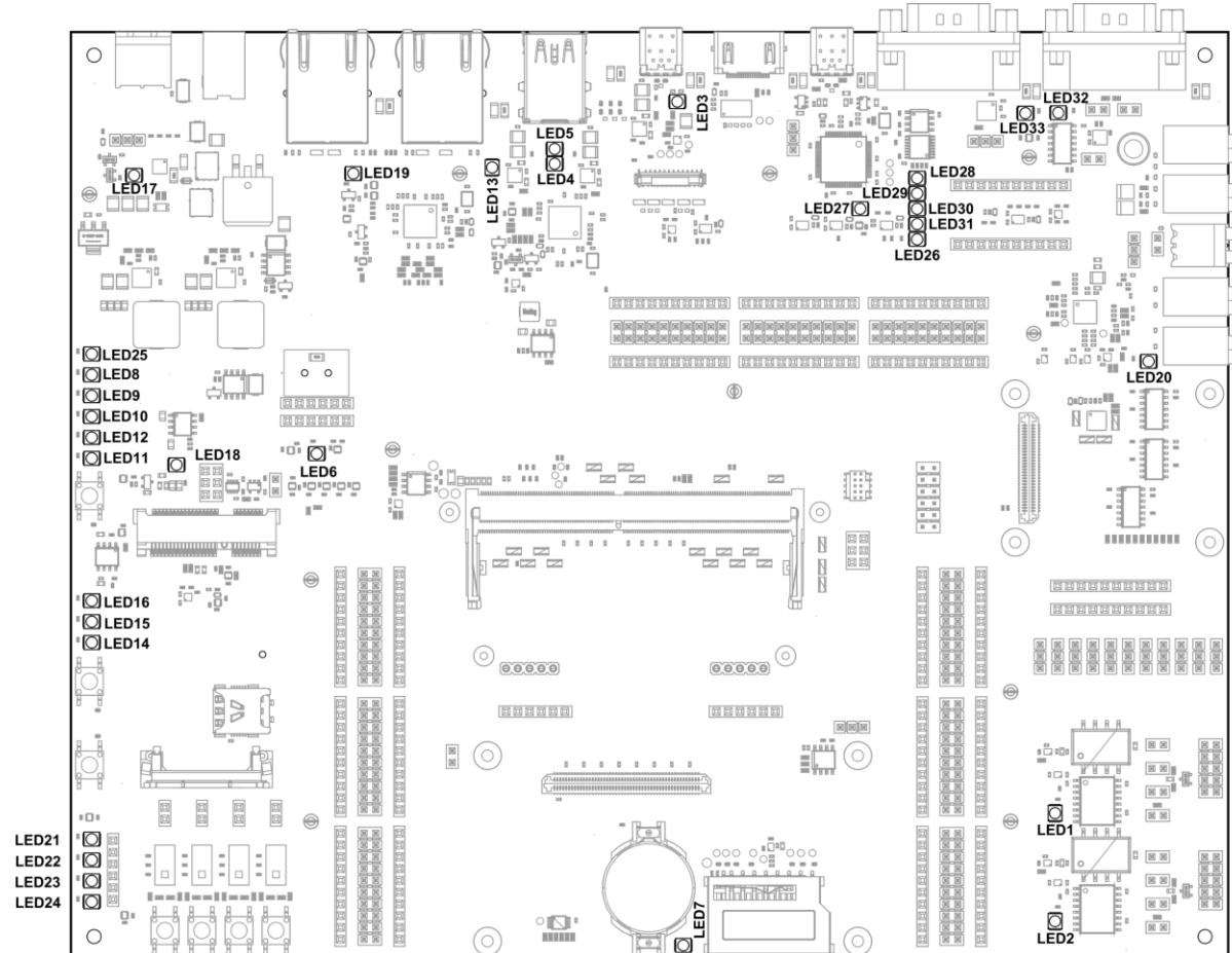
Figure 5: Indicator LEDs
