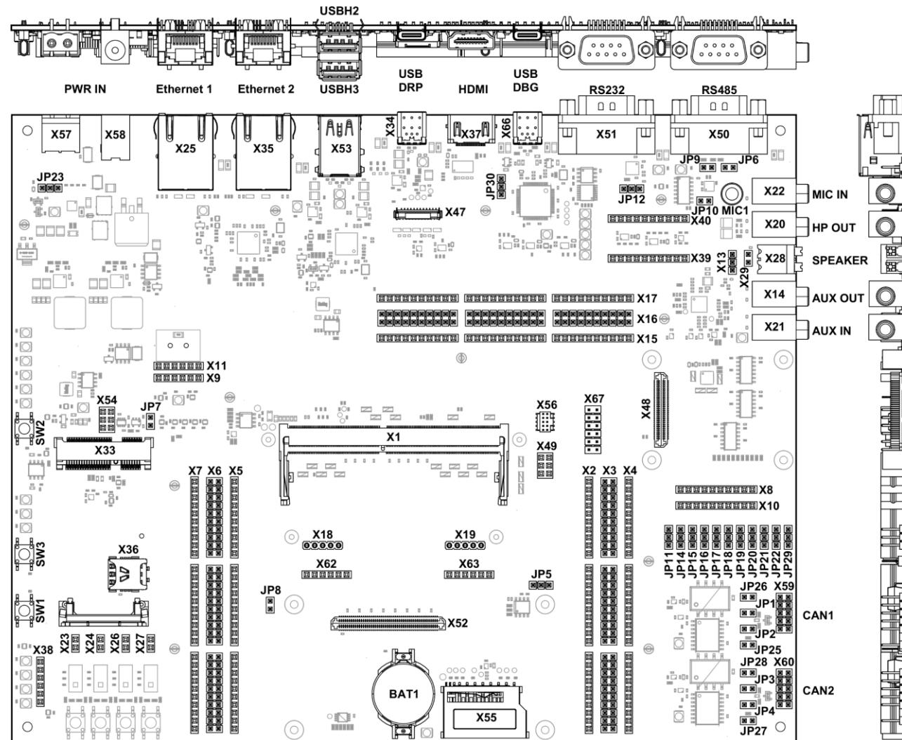
Figure 2: Verdin Development Board connectors and controls
