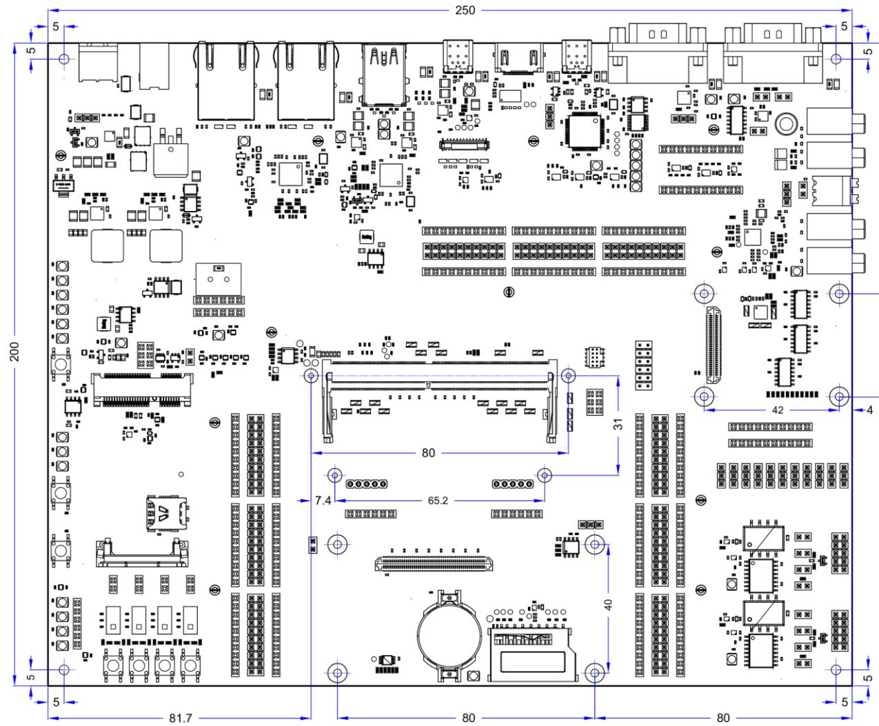
Figure 12: Verdin Development Board dimensions (in millimeters)
