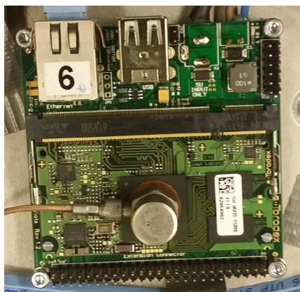
Resonance point at DUT No. 6: f=206.89\text{Hz}
