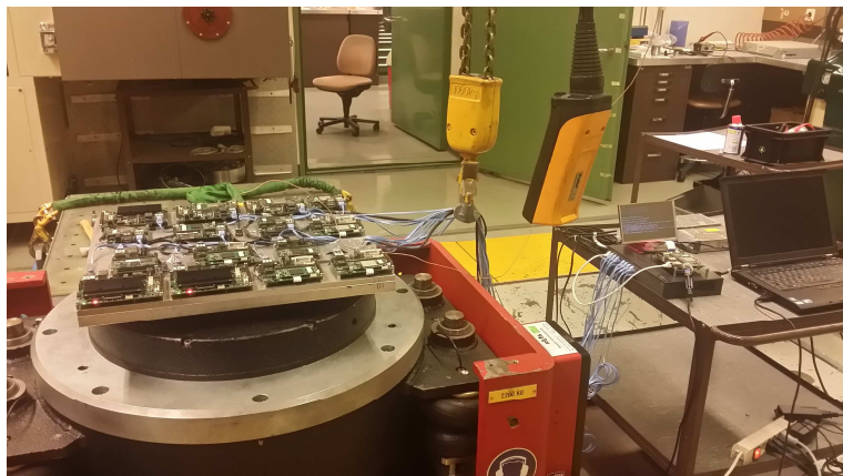
Resonance point at module 14: f=231\text{Hz}
