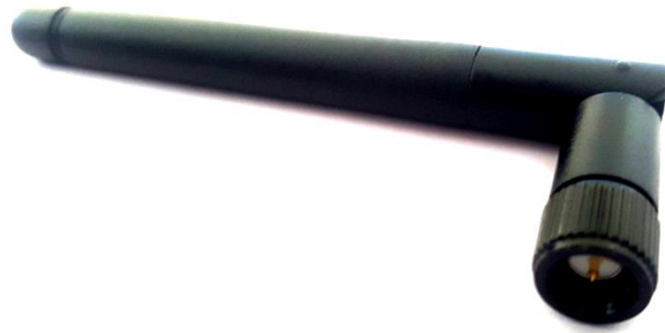
Figure 4: WADB-2458-23-SMAM showing SMA Plug (SMA Male) connector
