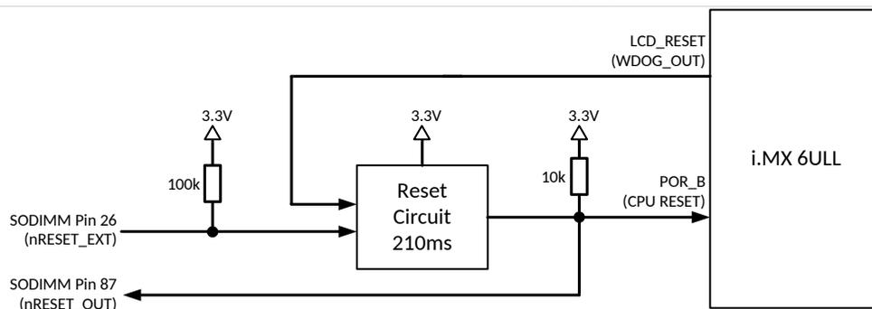
Figure 7: Reset Circuit
