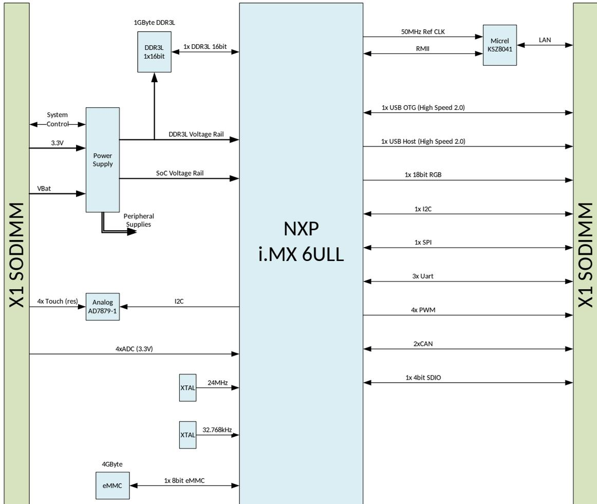
Figure 2 Colibri iMX6ULL 1GB IT Block Diagram
