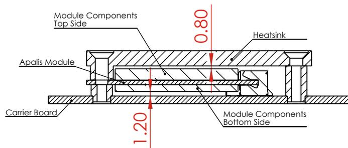
Figure 124: Maximum height of carrier board components under the module
