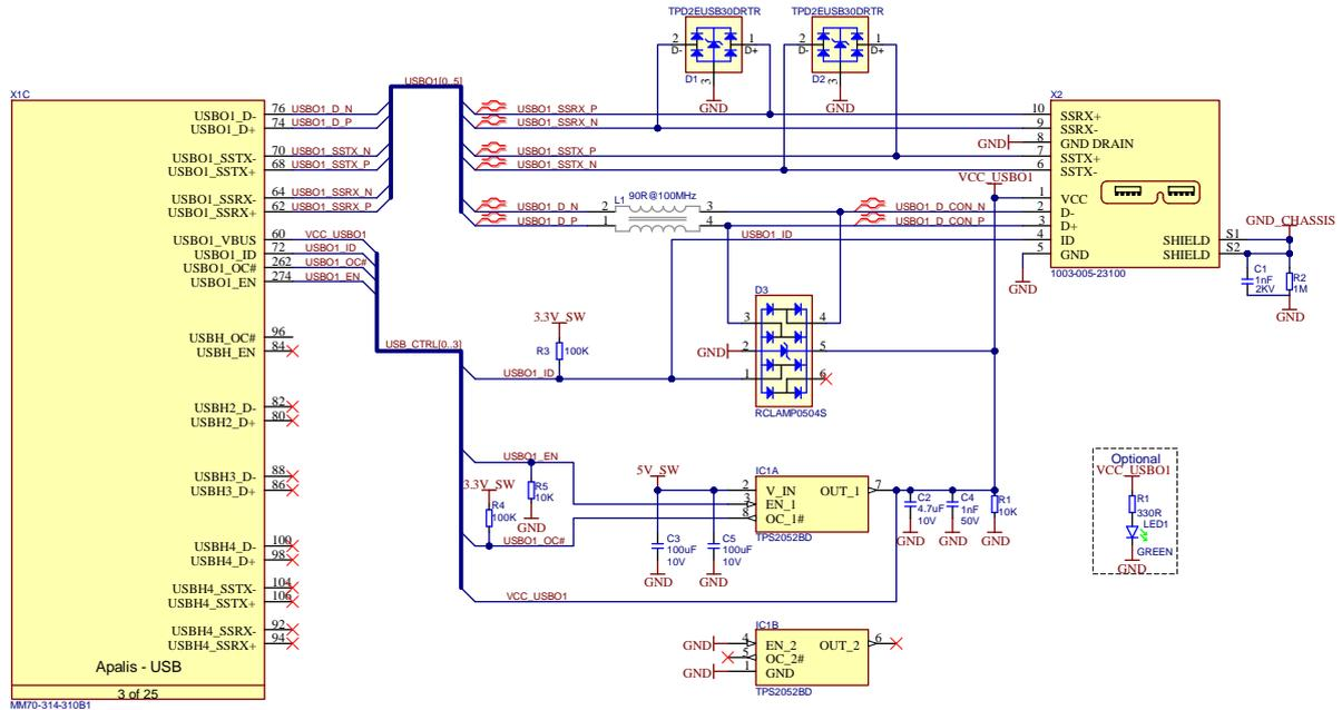
Figure 32: USB 3.x OTG (with Type Micro-AB connector) reference schematic
