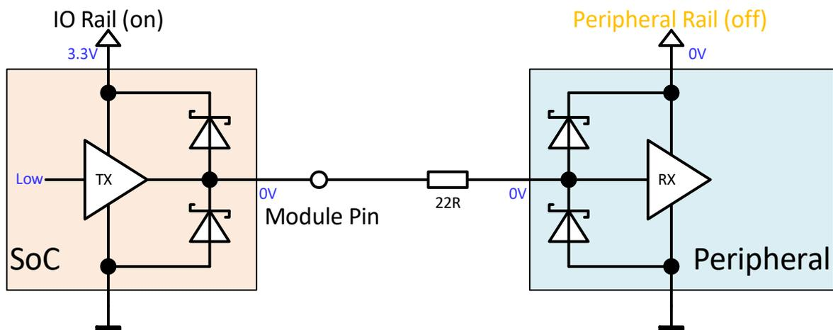
Figure 92: Make sure outputs are not driven high
