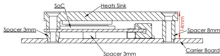
Figure 115: Stacking height of heat sink
