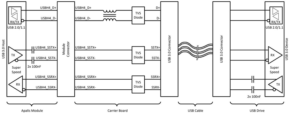
Figure 37: USB 3.x Host-Only (with Type-A connector) block diagram
