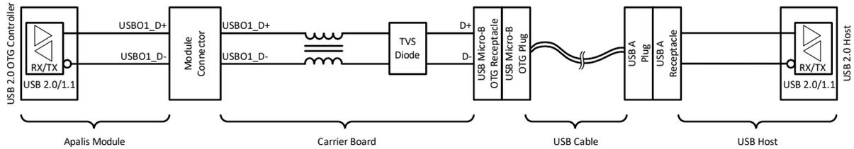
Figure 29: USB 2.0 OTG (with Type Micro-AB connector) block diagram
