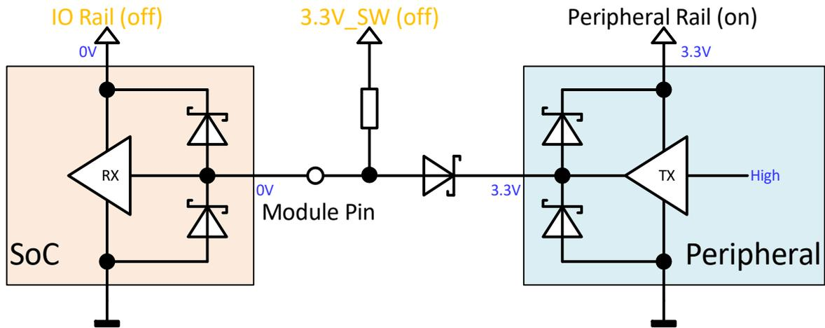
Figure 99: Diode circuit for backfeeding prevention with an external pull-up resistor
