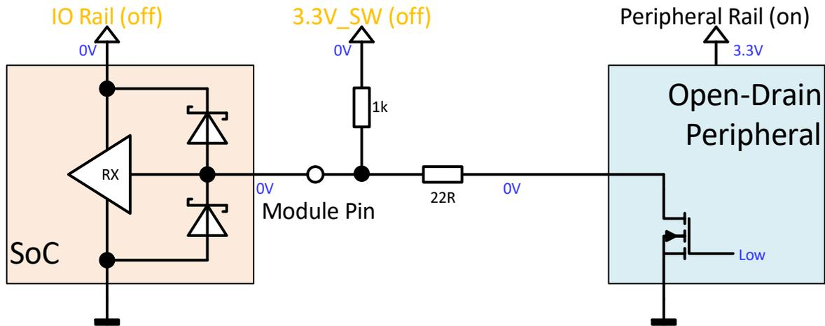
Figure 95: Correct pull-up rail for open-drain signals
