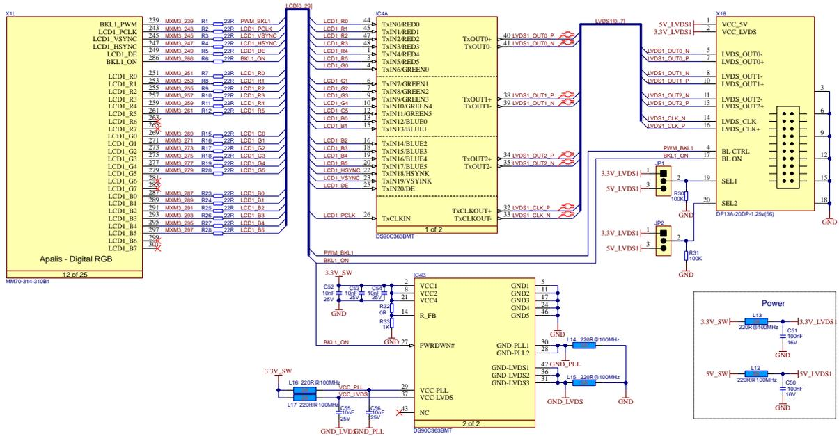
Figure 49: LVDS transmitter reference schematic
