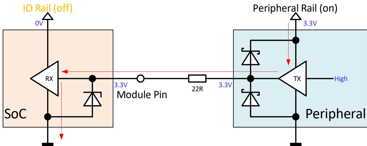
Figure 93: Input without backfeeding path
