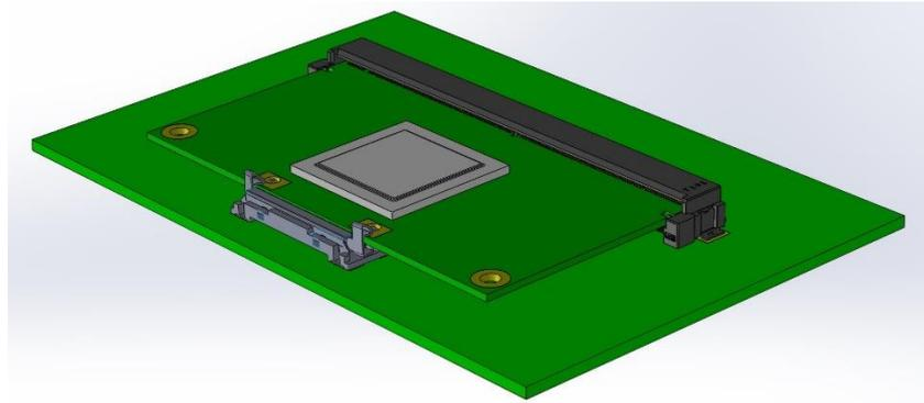
Figure 111: SnapLock fixation
