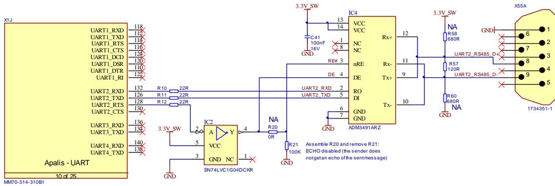
Figure 64: RS485 Reference Schematic
