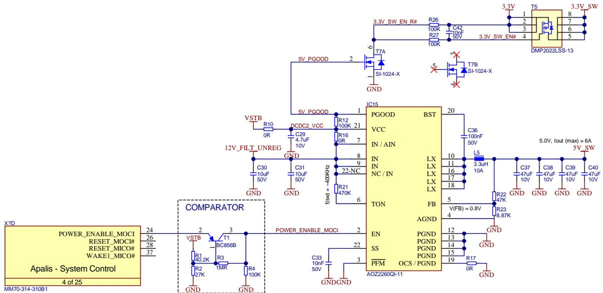
Figure 82: Simple POWER\_ENABLE\_MOCI comparator circuit
