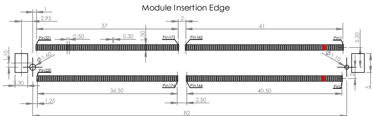
Figure 119: Module connector land pattern (dimensions in mm)
