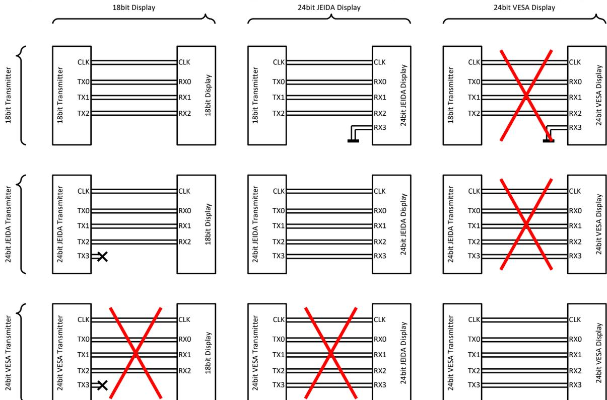
Figure 51: Compatibility between LVDS color mapping
