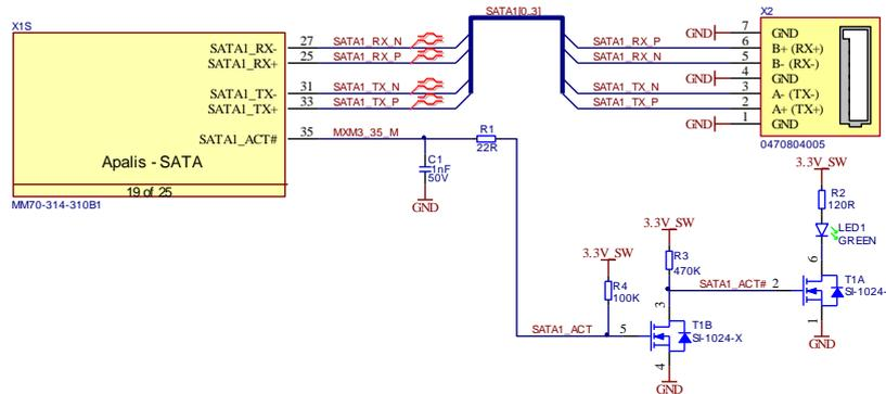
Figure 13: SATA connector reference schematic
