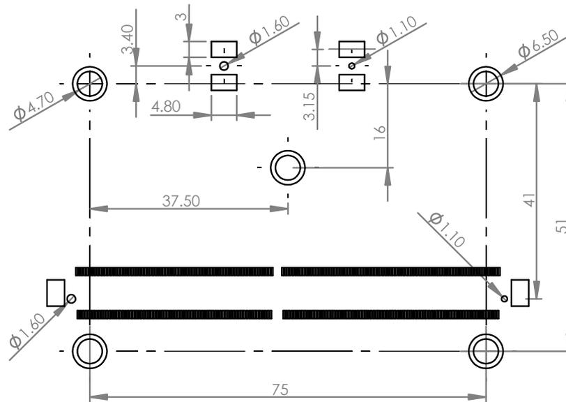
Figure 118: SnapLock and standoff land pattern (dimensions in mm)
