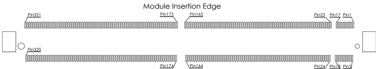
Figure 4: Pin numbering schema on the module connector land pattern
