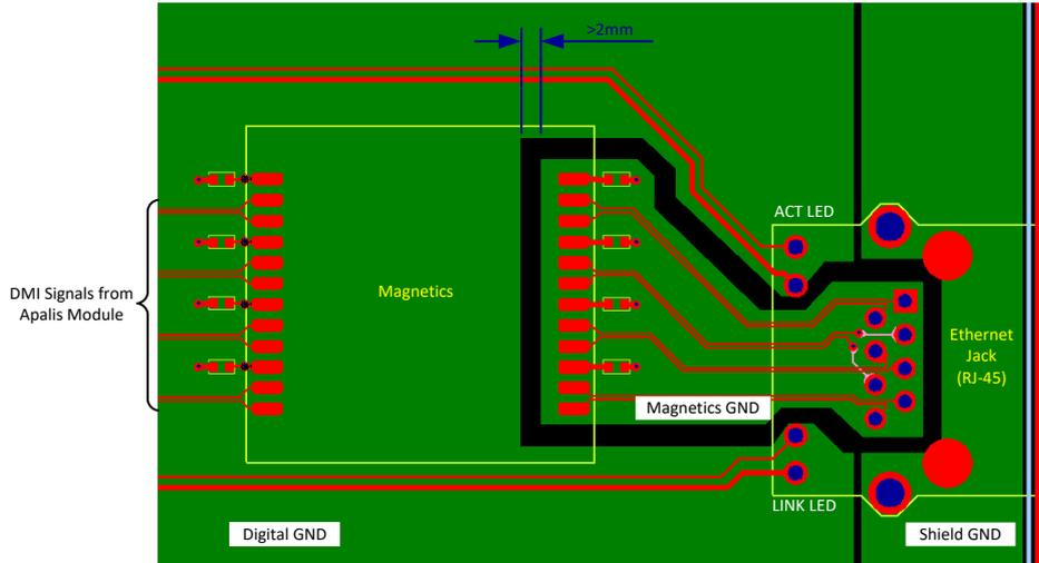
Figure 17: Separation of magnetics ground
