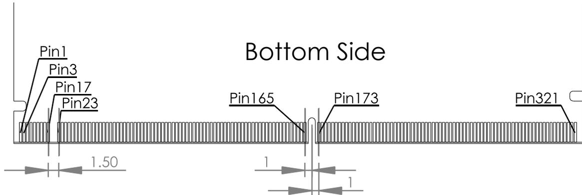
Figure 3: Pin numbering schema on the bottom side of the module
