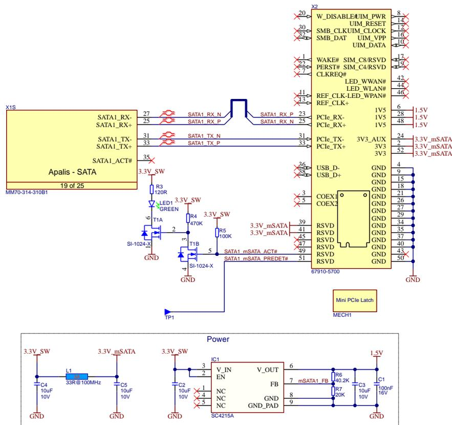
Figure 15: mSATA reference schematic
