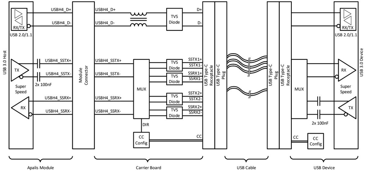
Figure 35: USB-C SuperSpeed DFP-Only (with Type-C connector) block diagram
