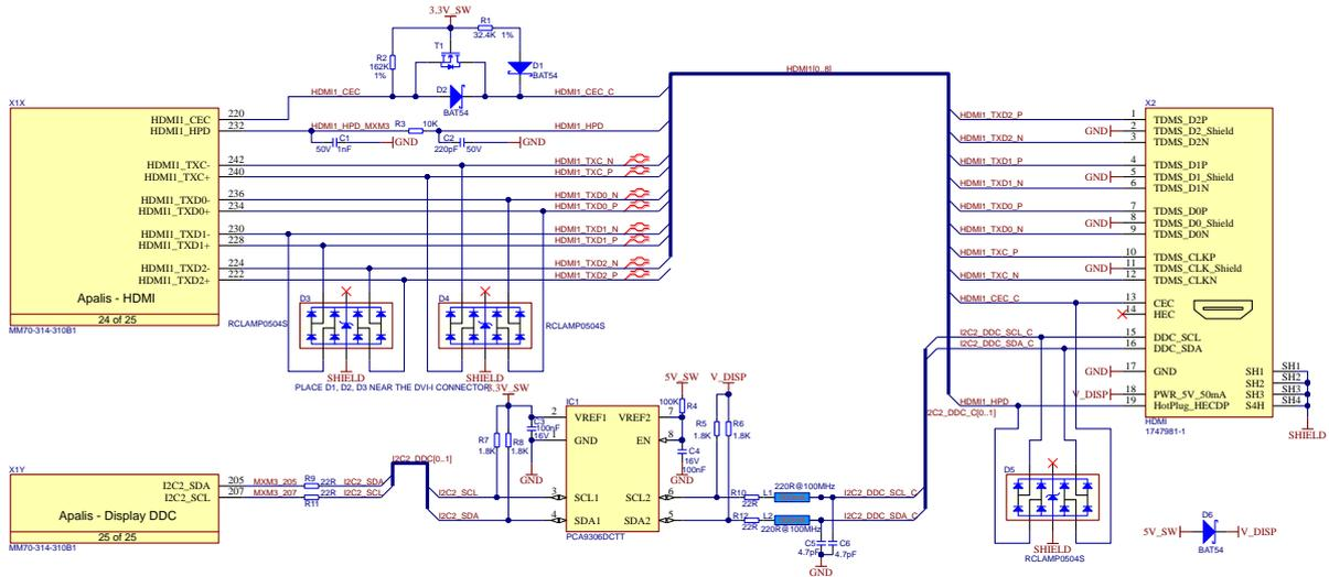
Figure 57: HDMI reference schematic
