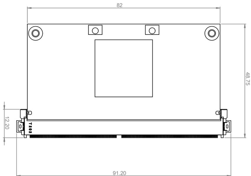
Figure 121: Minimum carrier board space requirement (dimensions in mm)
