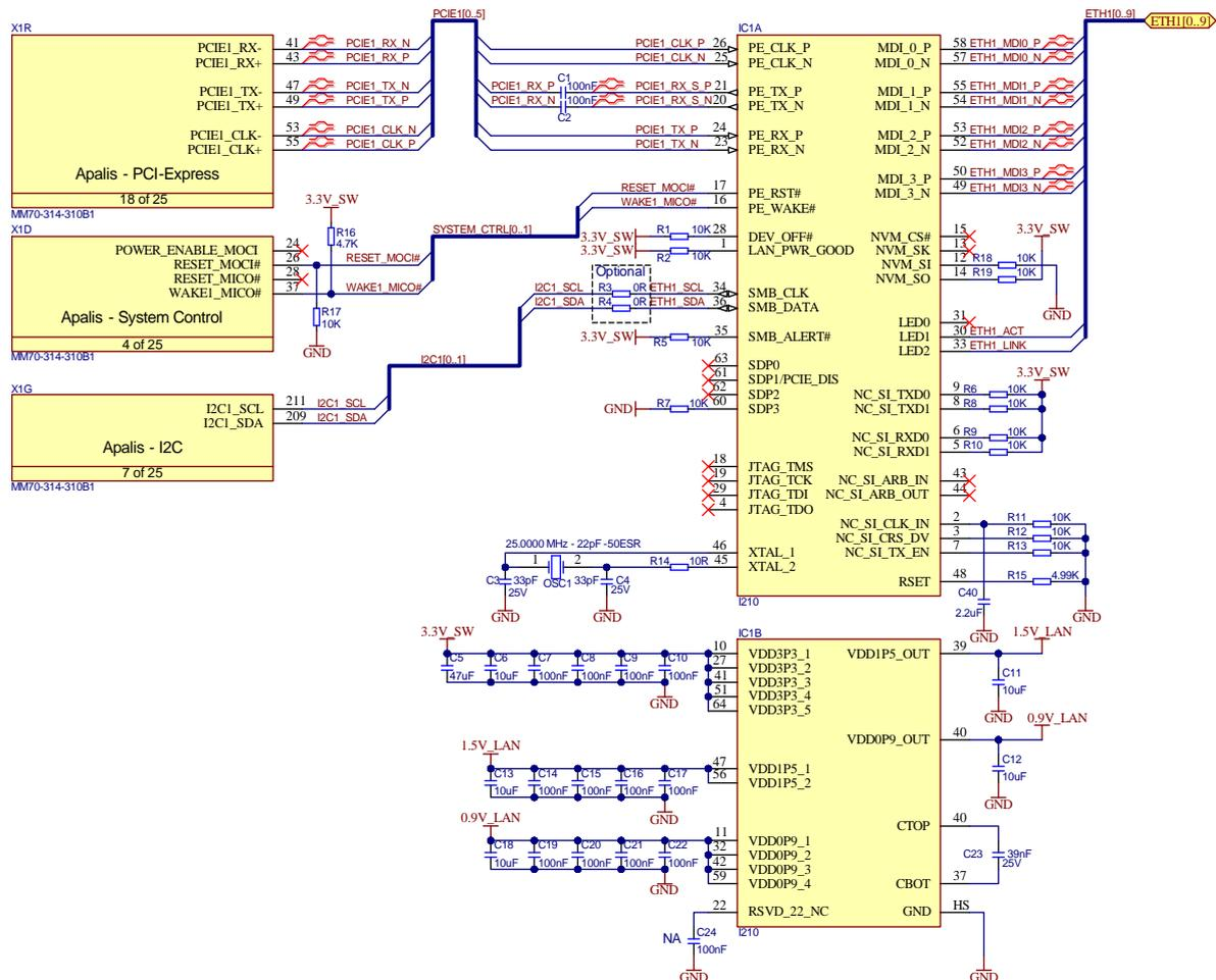
Figure 11: PCIe Device-Down example schematic
