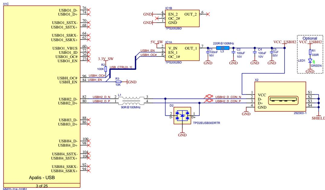
Figure 40: USB 2.0 Host-Only (with Type-A connector) reference schematic
