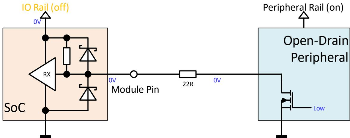
Figure 96: Using internal pull-up resistor
