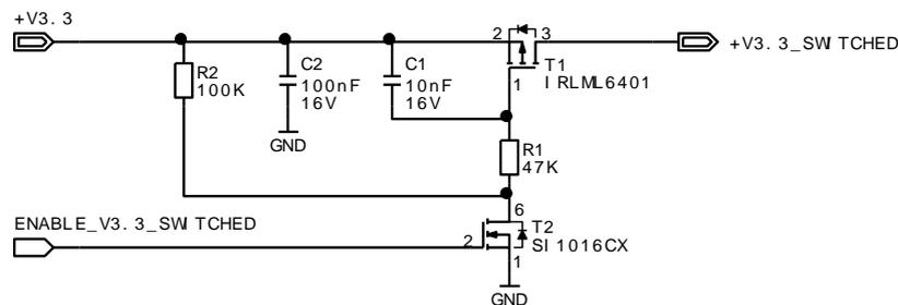
Figure 80: Simple voltage switch circuit
