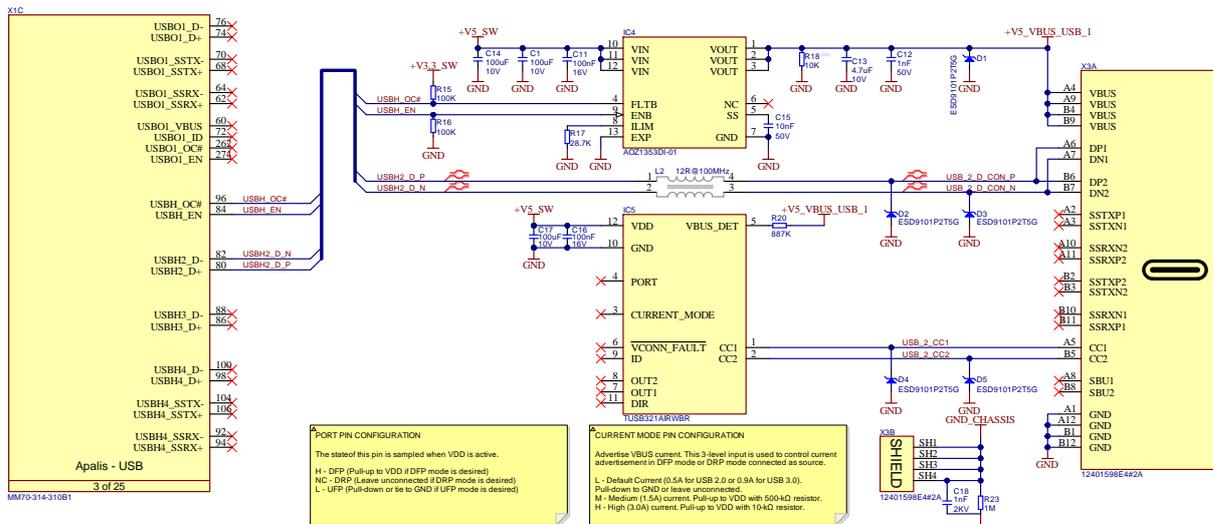
Figure 34: USB-C High-Speed DFP-Only (with Type-C connector) reference schematic
