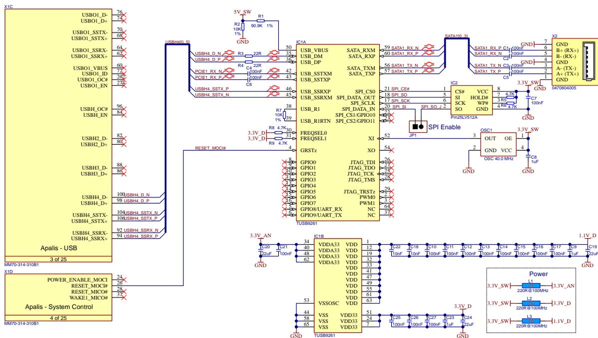
Figure 46: USB 3.x device down reference schematic (USB3.x to SATA Bridge)
