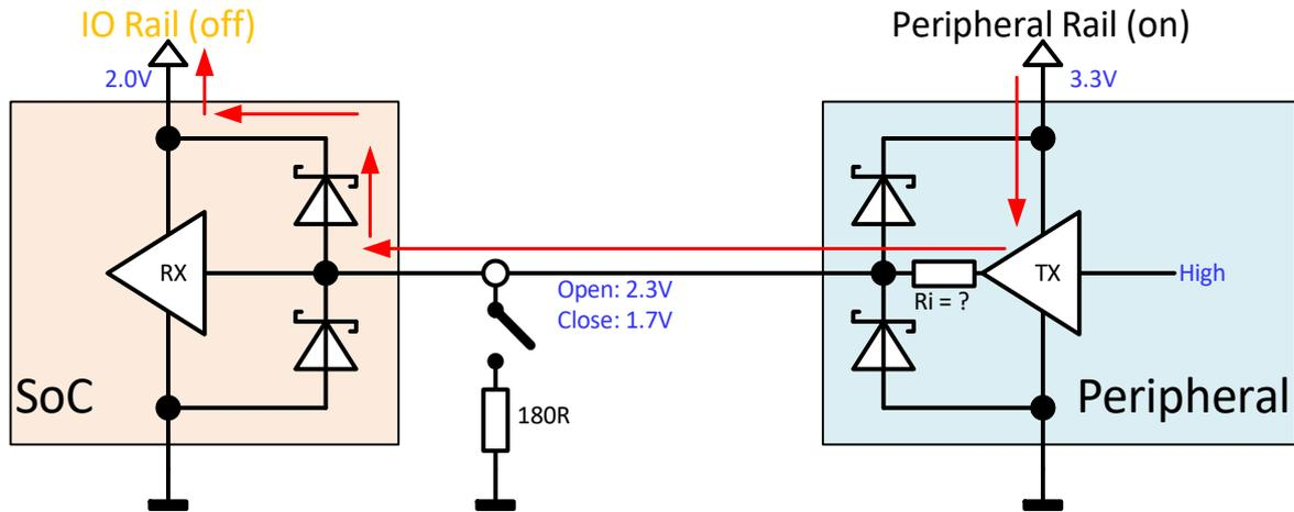
Figure 89: Evaluating the internal resistance of the driver
