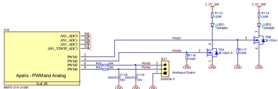
Figure 67: PWM Example Schematic
