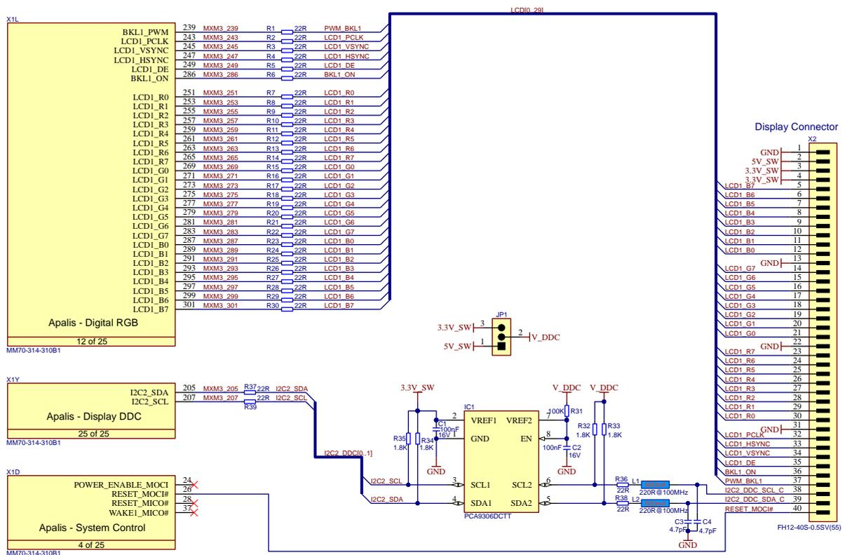
Figure 47: 24-bit parallel RGB display reference schematic
