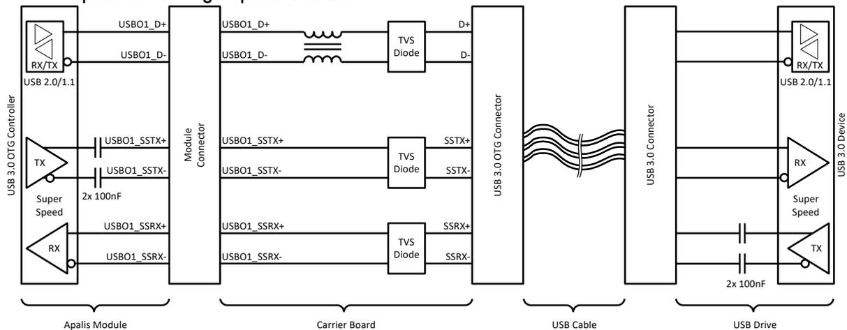
Figure 31: USB 3.x OTG (with Type Micro-AB connector) block diagram
