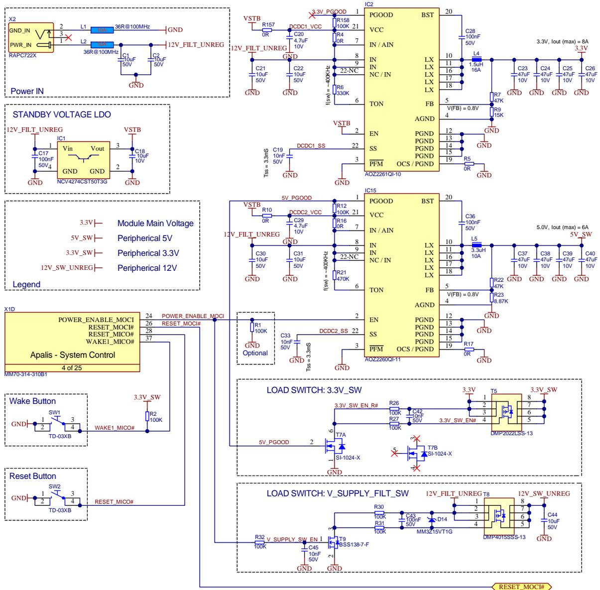
Figure 81: Simple power supply reference schematic
