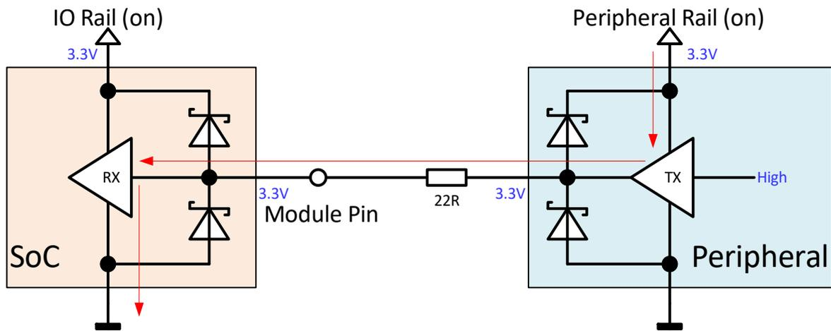
Figure 83: SoC input pin with ESD protection, both power rails on
