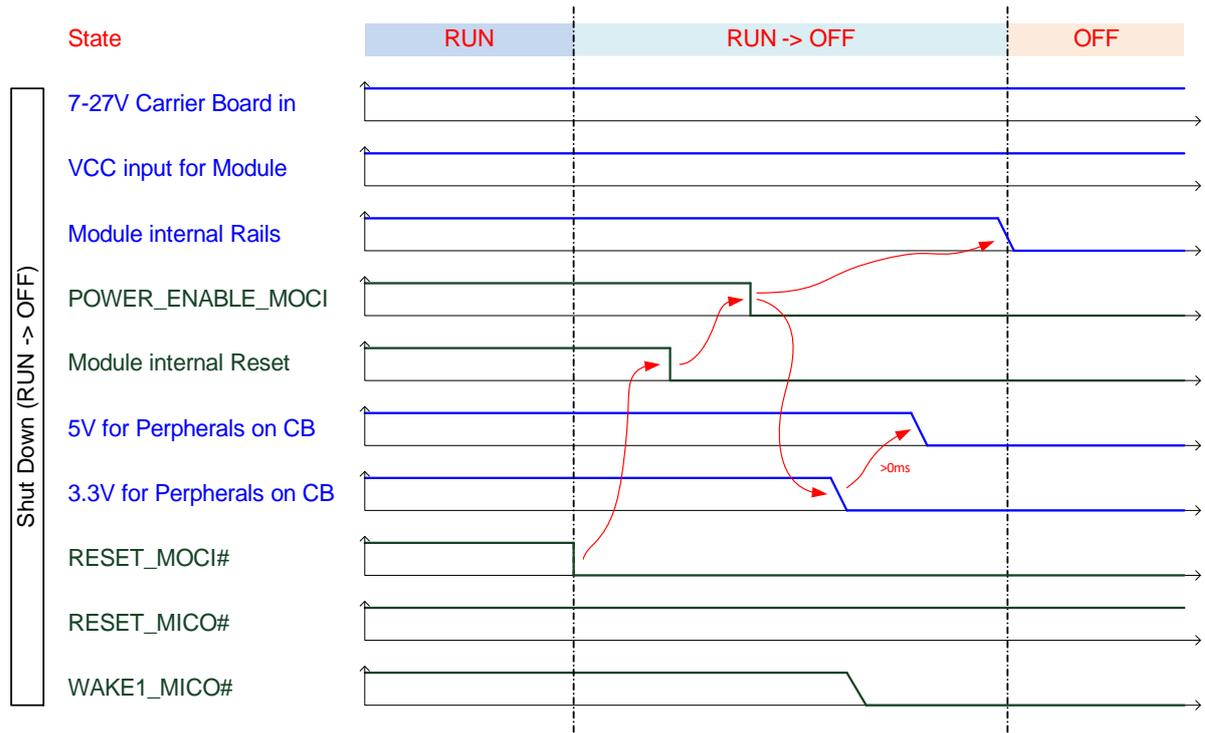
Figure 75: Shut-down sequence
