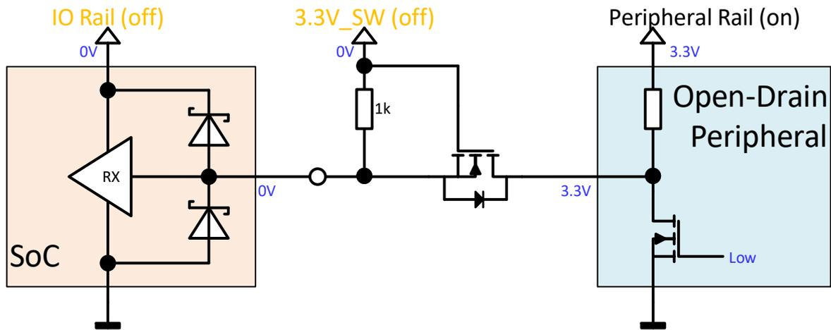
Figure 97: Simple FET circuit for open-drain signals
