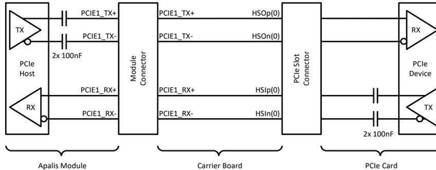
Figure 6: PCIe x1 Slot Block Diagram
