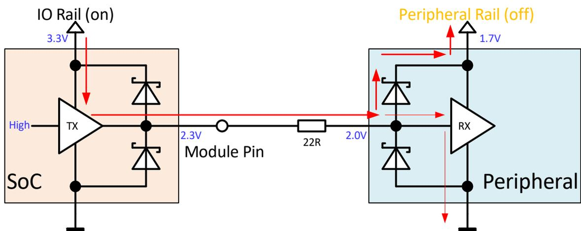
Figure 86: Backfeeding to peripherals
