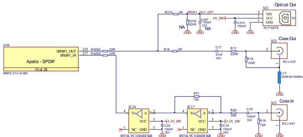
Figure 70: S/PDIF Reference Schematic
