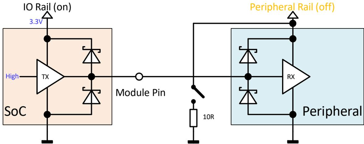
Figure 107: Additional load on the peripheral rail
