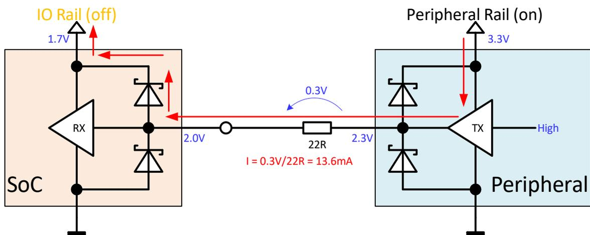
Figure 88: Measuring backfeeding current
