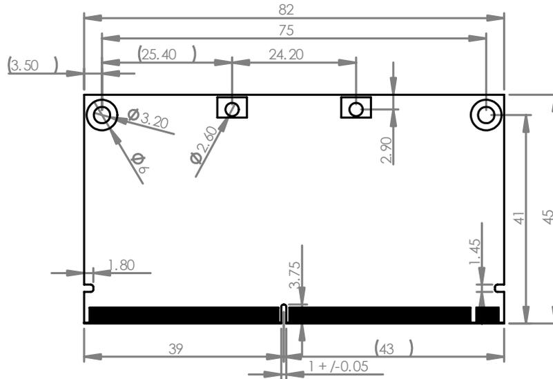
Figure 116: Module dimension top side (dimensions in mm)
