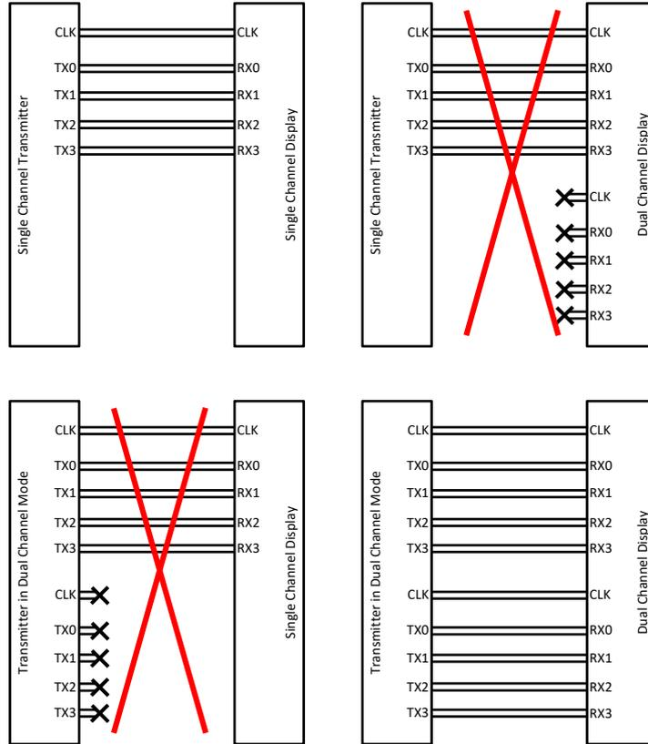
Figure 50: Compatibility between Single and Dual Channel LVDS
