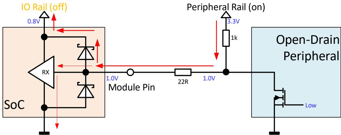
Figure 85: Backfeeding with open-drain signals
