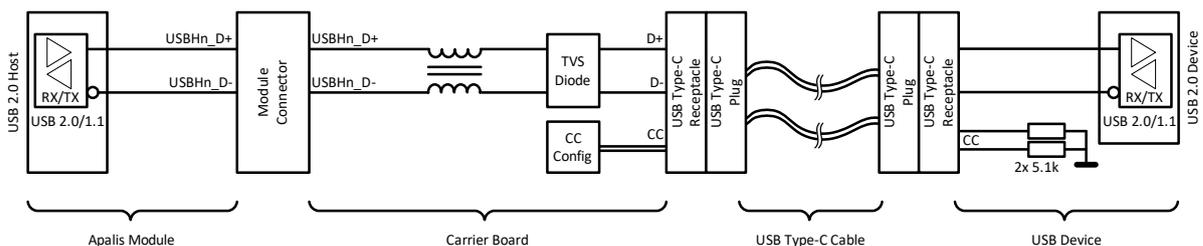
Figure 33: USB-C High-Speed DFP-Only (with Type-C connector) block diagram
