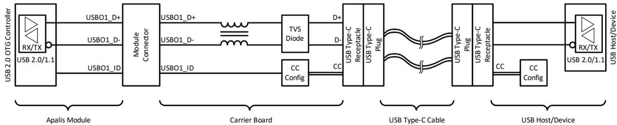
Figure 25: USB-C High-Speed Dual Role (with Type-C connector) block diagram
