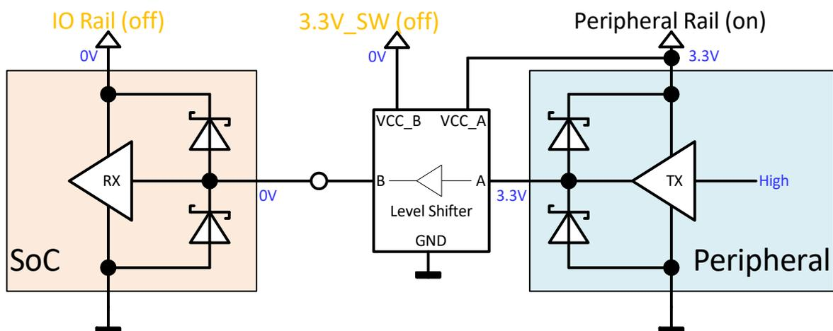
Figure 104: Level shifter for preventing backfeeding
