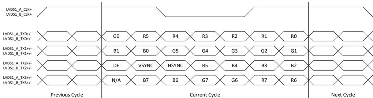
Figure 54: 24-bit VESA LVDS color mapping
