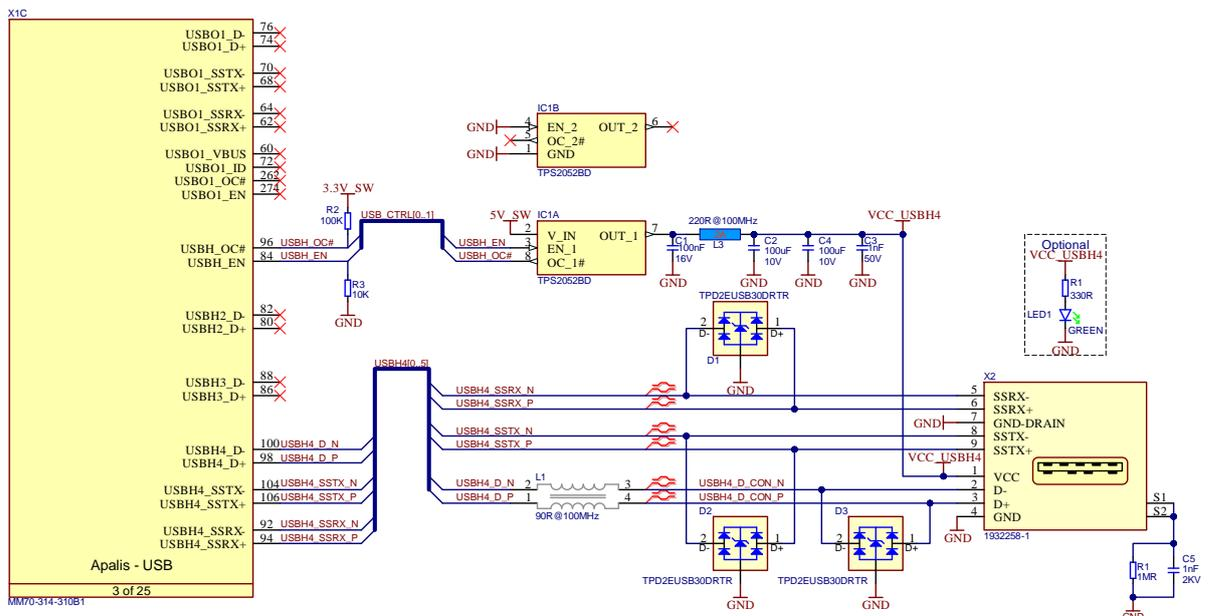
Figure 38: USB 3.x Host-Only (with Type-A connector) reference schematic
