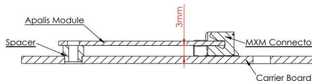
Figure 109: Board Stacking Height
