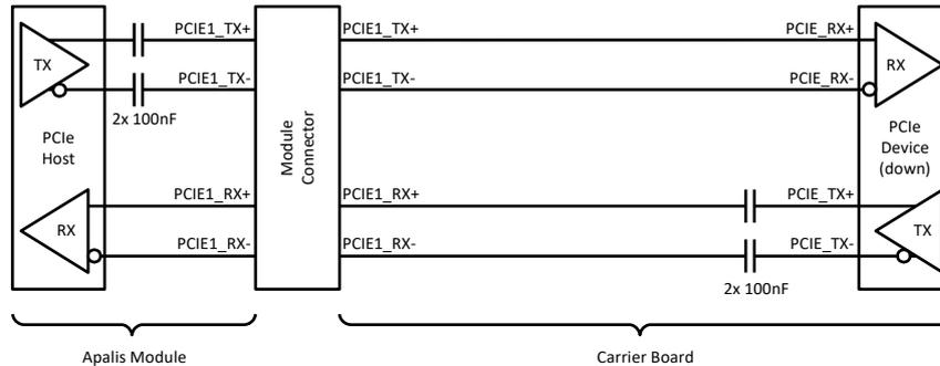
Figure 10: PCIe Device-Down block diagram
