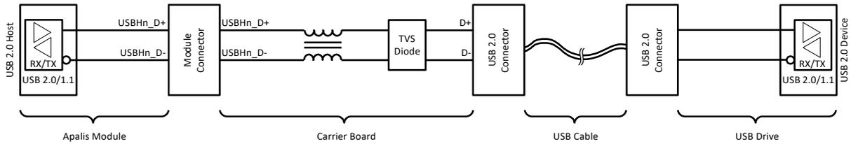
Figure 39: USB 2.0 Host-Only (with Type-A connector) block diagram
