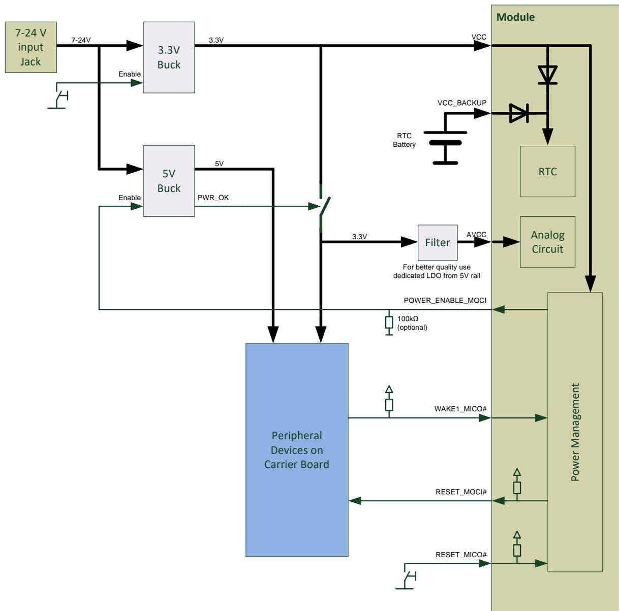
Figure 72: Power Block Diagram
