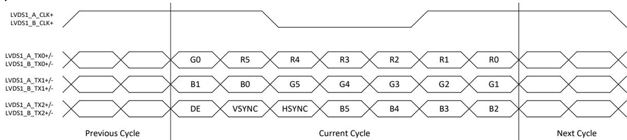
Figure 52: 18-bit LVDS Color Mapping
