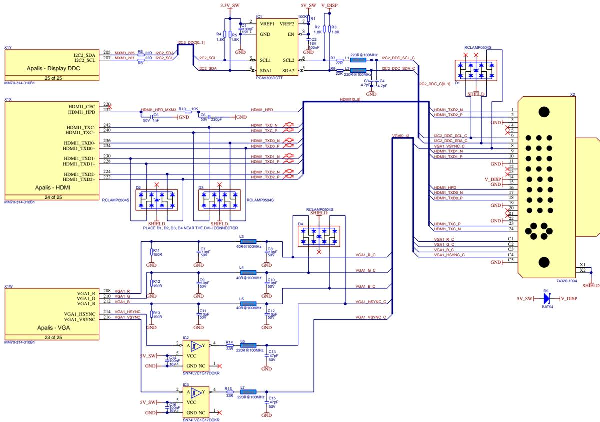
Figure 56: DVI-I reference schematic
