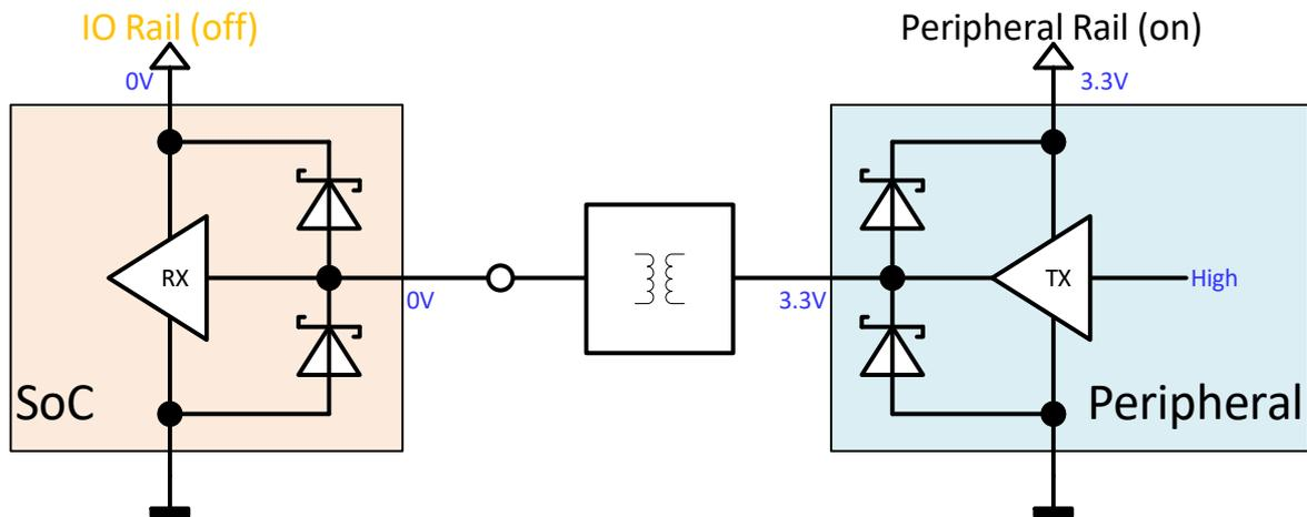
Figure 105: Galvanic isolation between input and output
