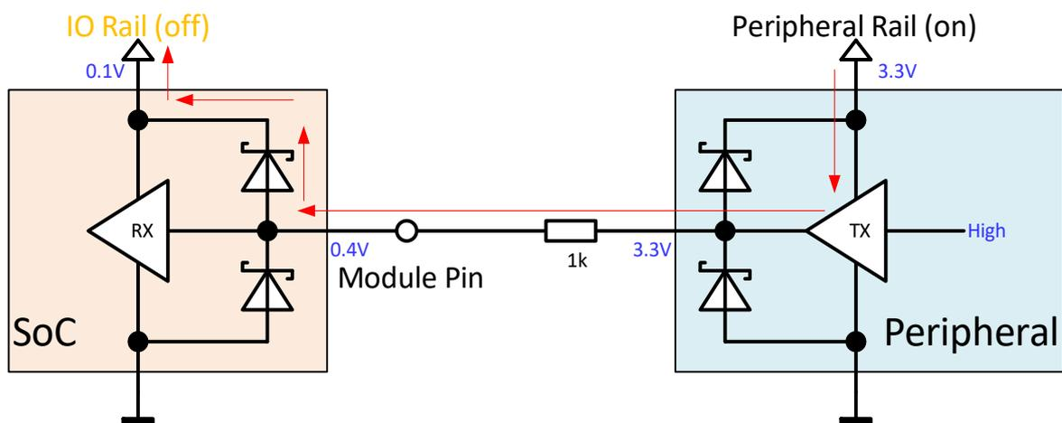
Figure 94: Series resistor for limiting backfeeding
