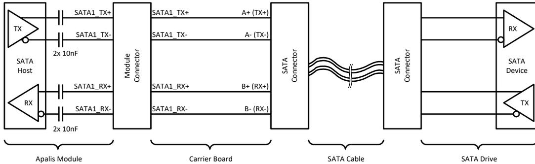
Figure 12: SATA connector block diagram
