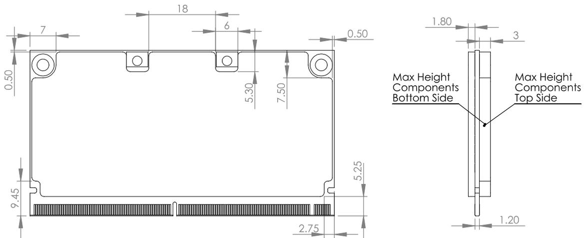
Figure 123: Maximum height of components on module (dimensions in mm)
