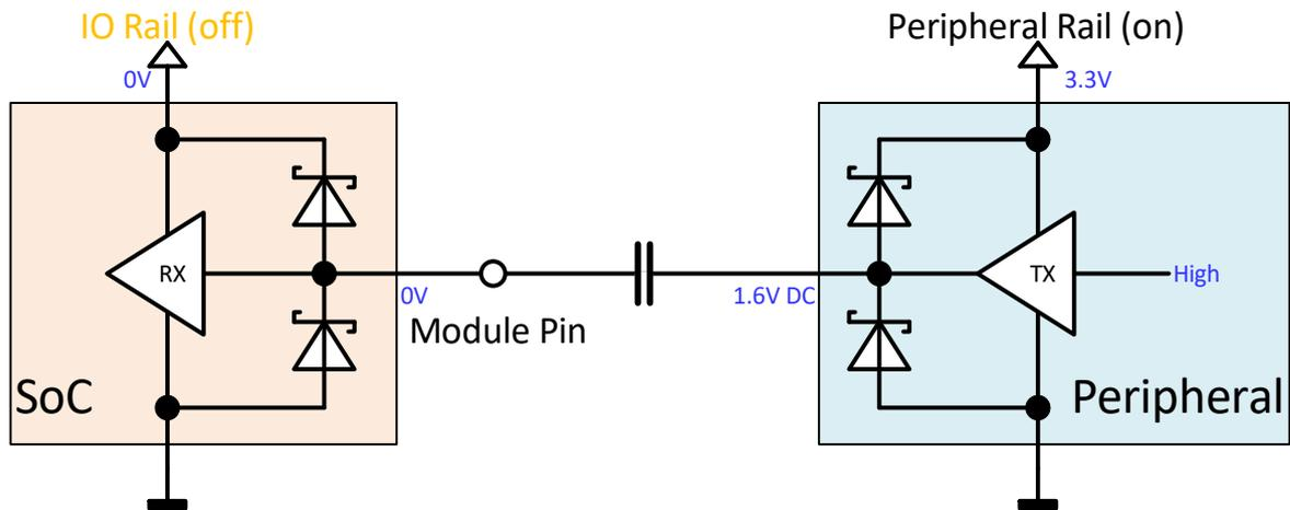
Figure 100: Capacitive coupled signals
