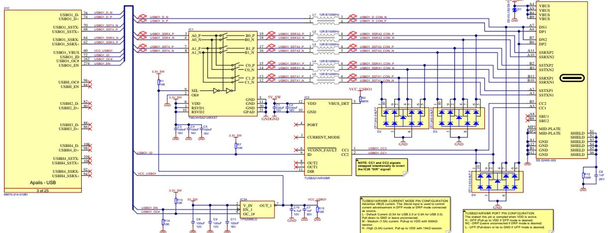
Figure 28: USB-C SuperSpeed Dual Role (with Type-C connector) reference schematic
