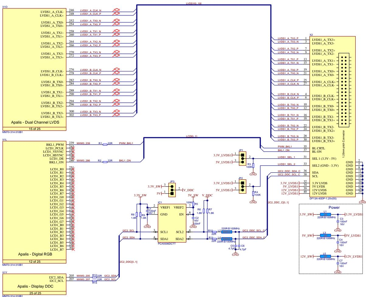
Figure 55: 24-bit Dual-channel LVDS display reference schematic
