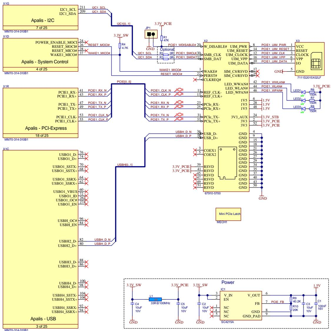
Figure 9: Mini PCIe card reference schematic
