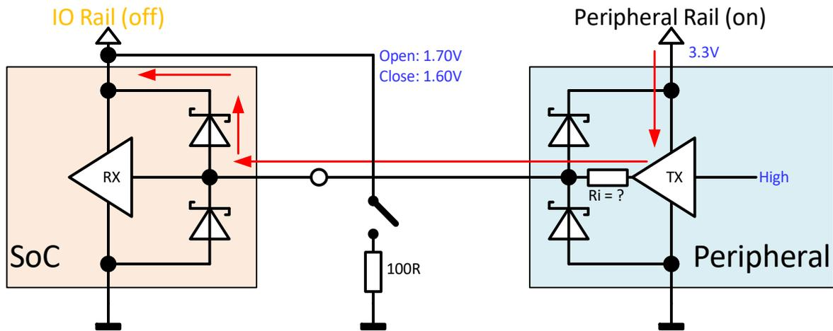
Figure 90: Evaluating the total internal resistance of the backfeeding
