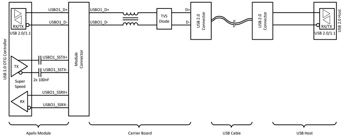
Figure 43: USB 2.0 Client-Only (with Type-B connector) block diagram
