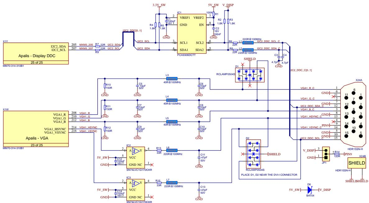
Figure 58: VGA reference schematic
