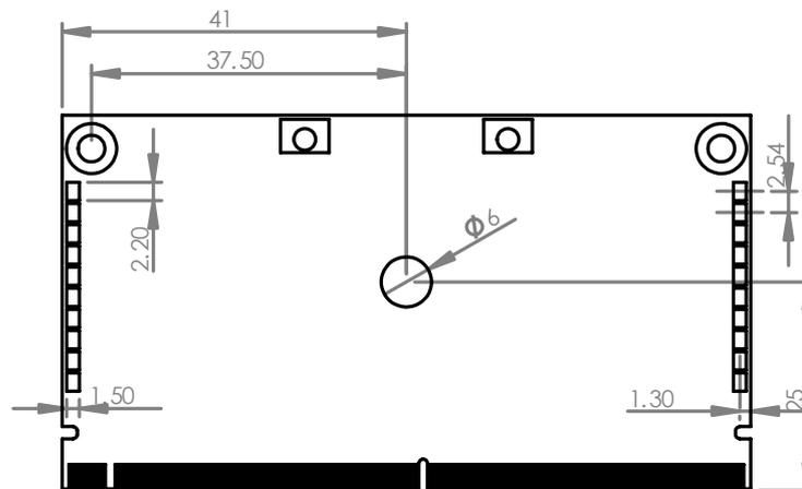
Figure 117: Module dimension bottom side (dimensions in mm)
