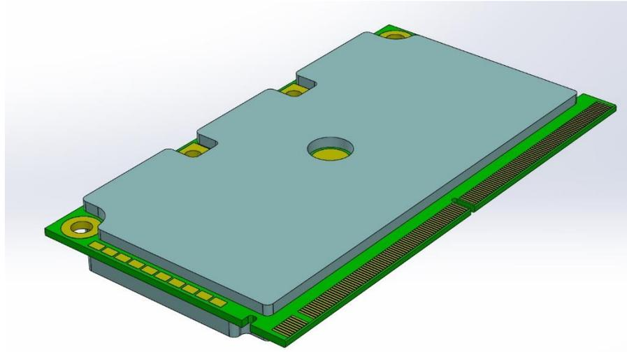
Figure 122: Maximum space requirement of components on module (bottom view)
