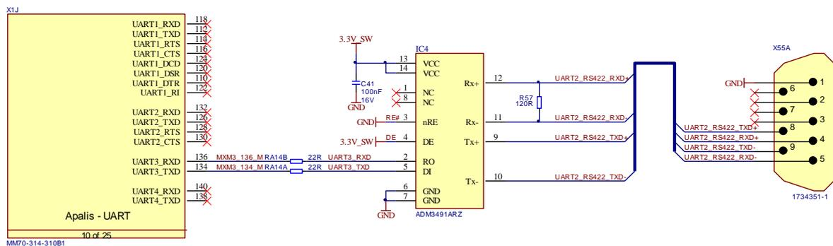
Figure 63: RS422 Reference Schematic
