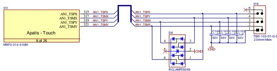
Figure 71: Touch Interface Reference Schematic
