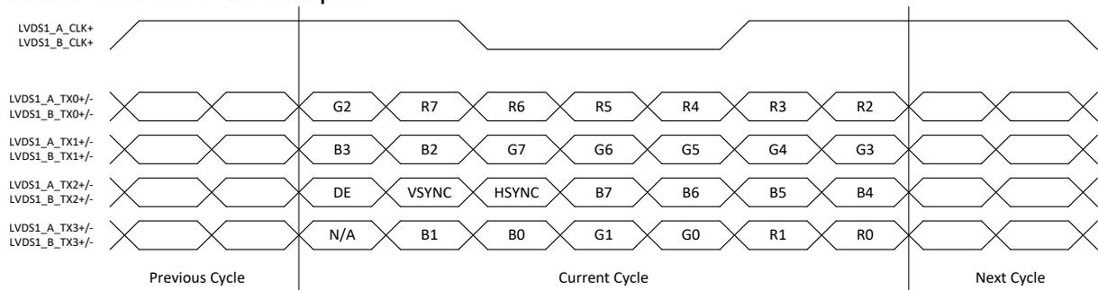
Figure 53: 24-bit JEIDA LVDS color mapping
