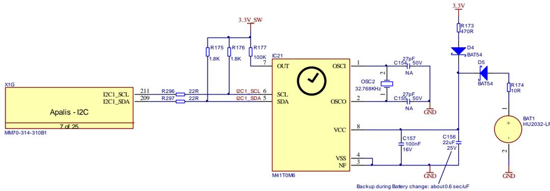
Figure 61: External RTC Reference Schematic
