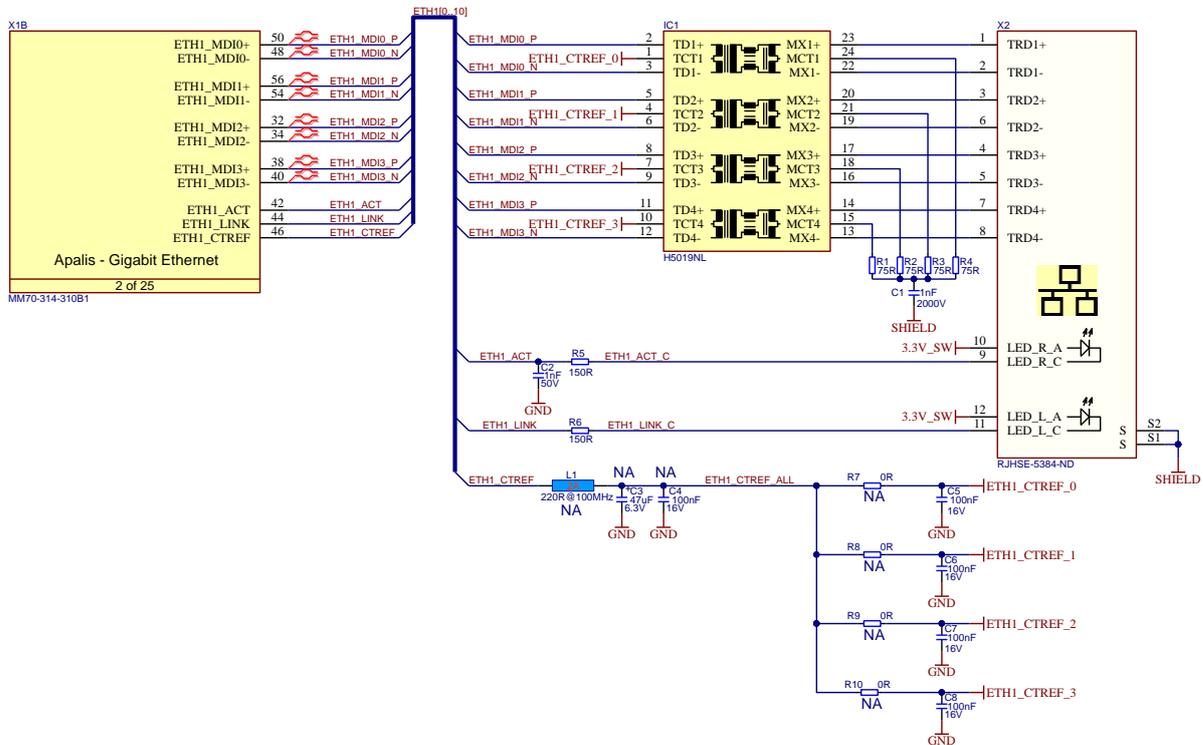
Figure 18: Gigabit Ethernet with discrete magnetics reference schematic
