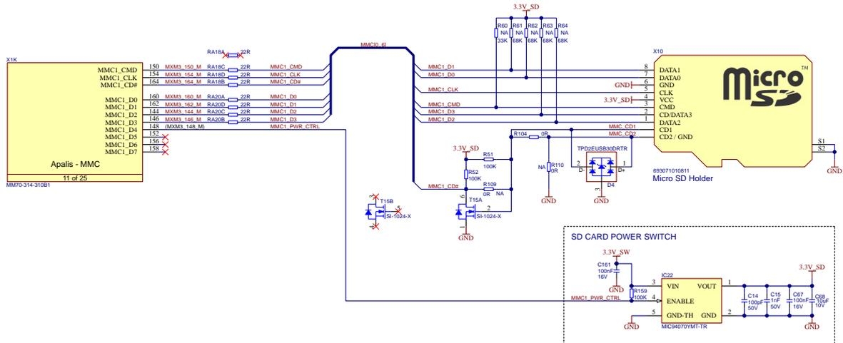
Figure 59: 4bit SD Card Slot Reference Schematic
