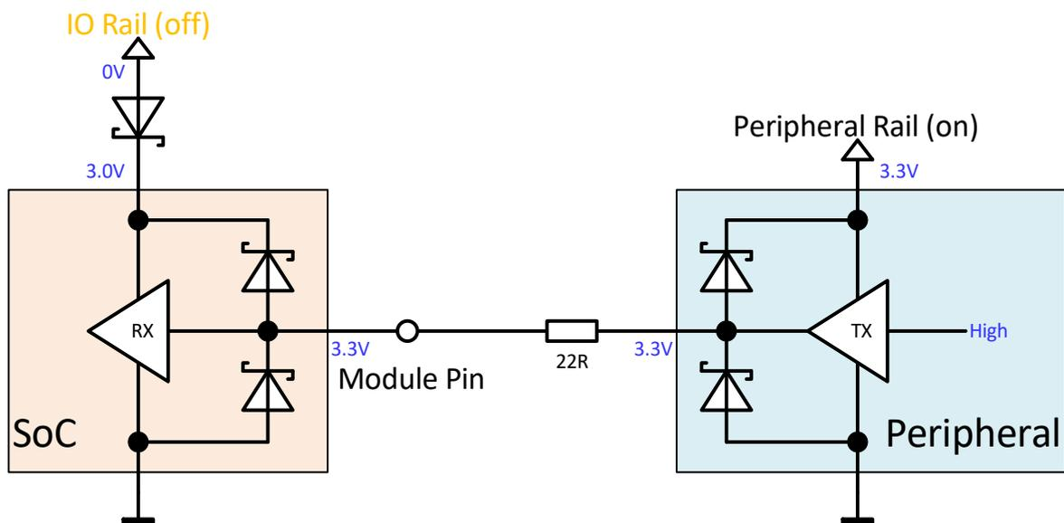
Figure 106: Reverse current protection diode
