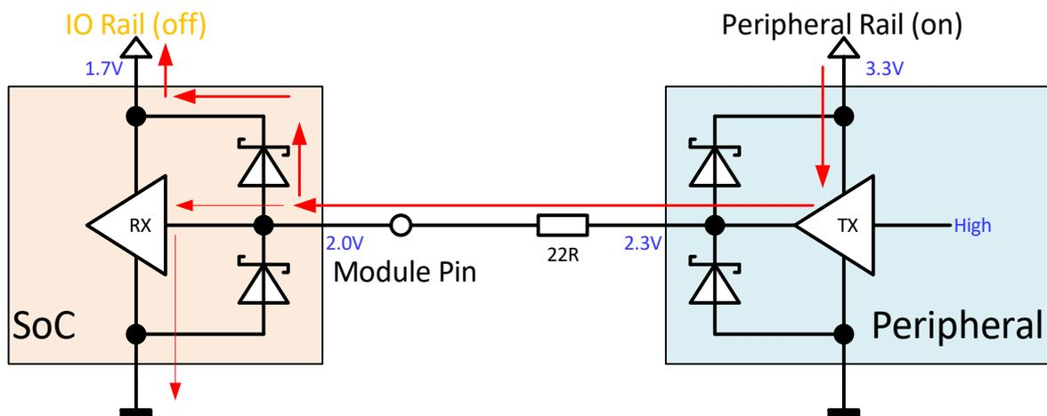
Figure 84: Backfeeding if IO rail is off and the peripheral signal is high
