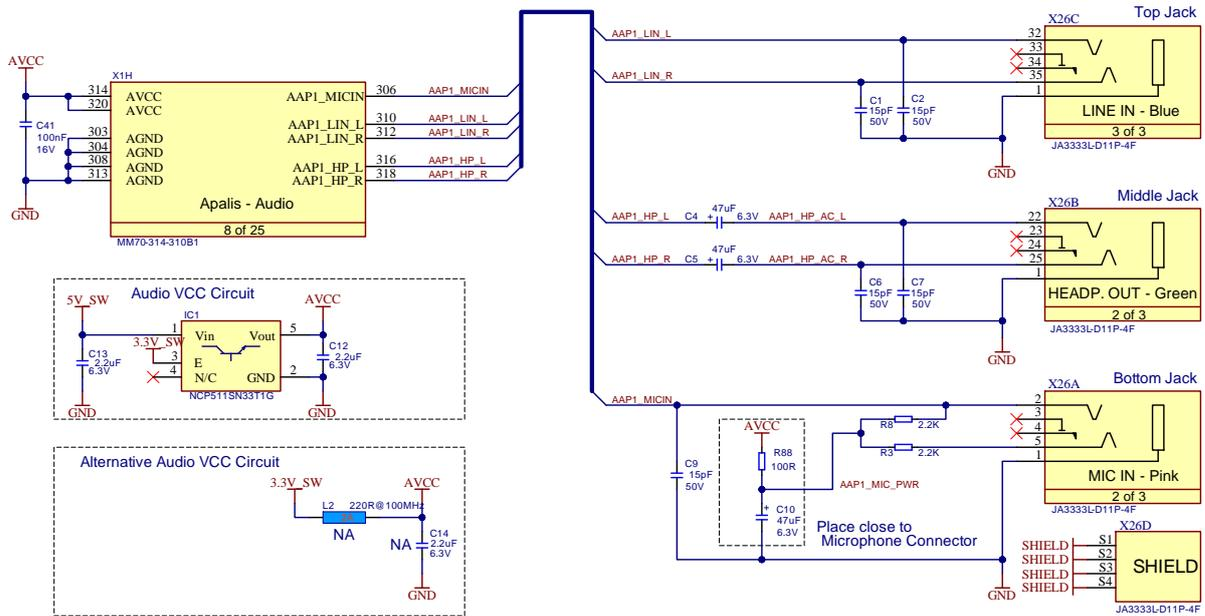
Figure 68: Analogue Audio Reference Schematic
