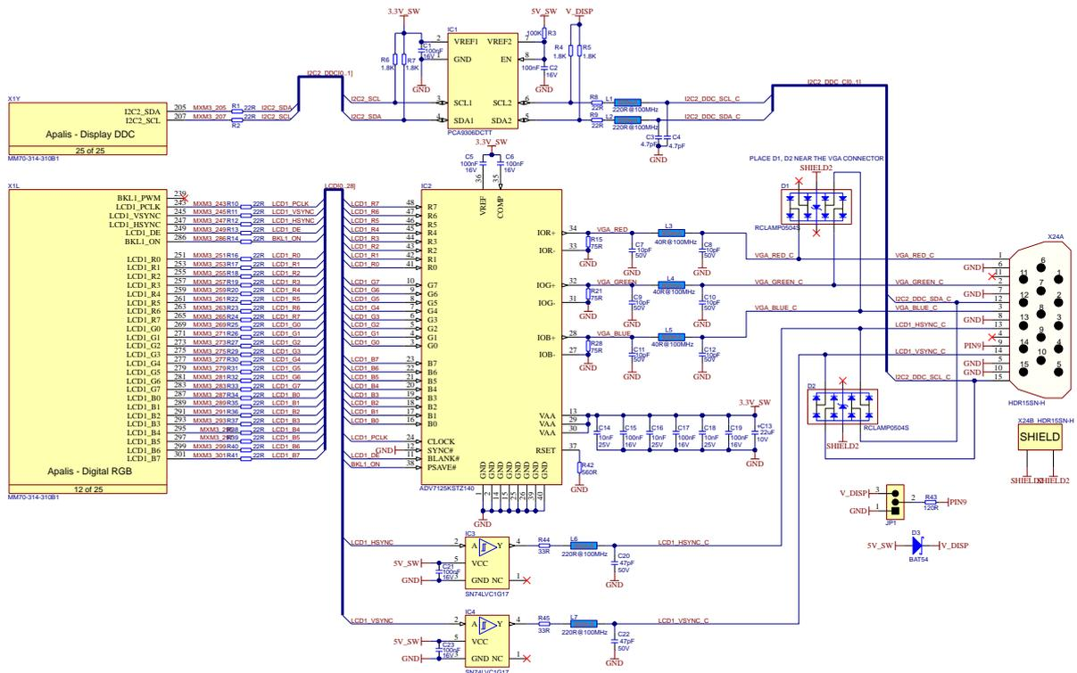
Figure 48: VGA DAC reference schematic
