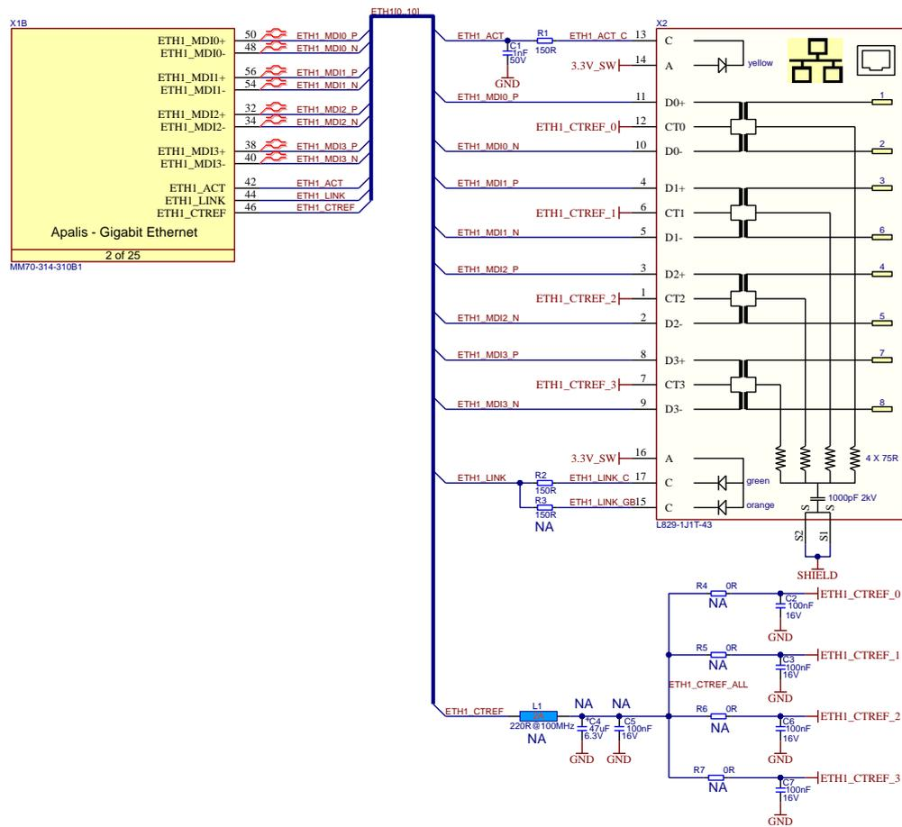
Figure 16: Gigabit Ethernet with integrated magnetics reference schematic
