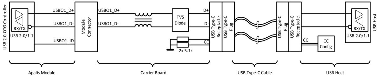
Figure 41: USB-C High-Speed UFP-Only (with Type-C connector) block diagram
