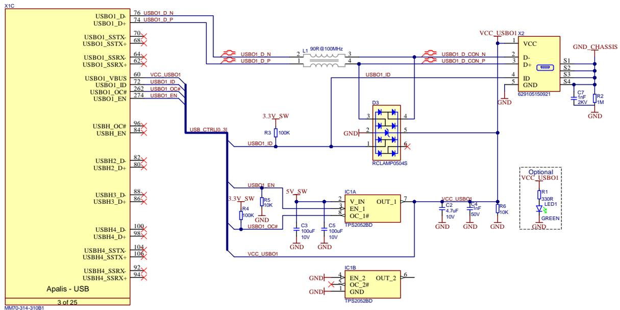
Figure 30: USB 2.0 OTG (with Type Micro-AB connector) reference schematic
