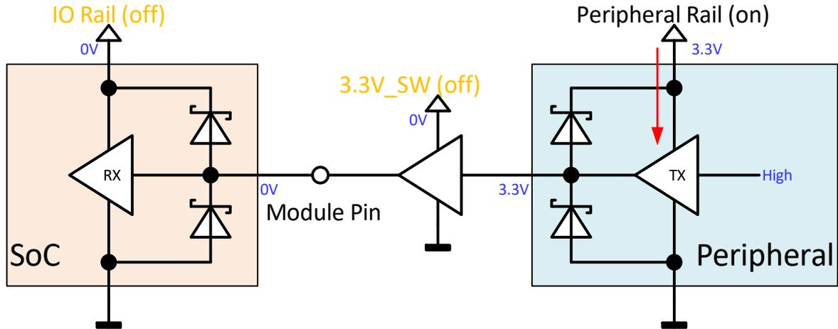
Figure 101: Non-backfeeding buffer
