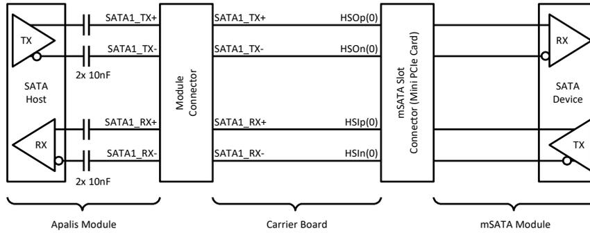
Figure 14: mSATA block diagram
