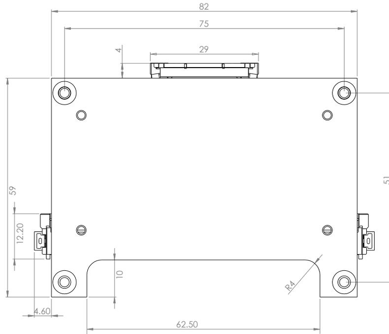
Figure 120: Maximum carrier board space requirement (dimensions in mm)
