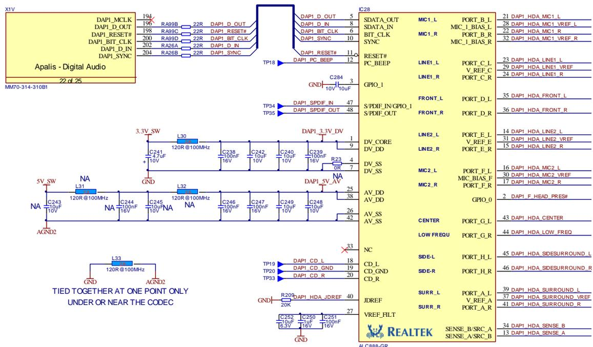
Figure 69: HDA Reference Schematic
