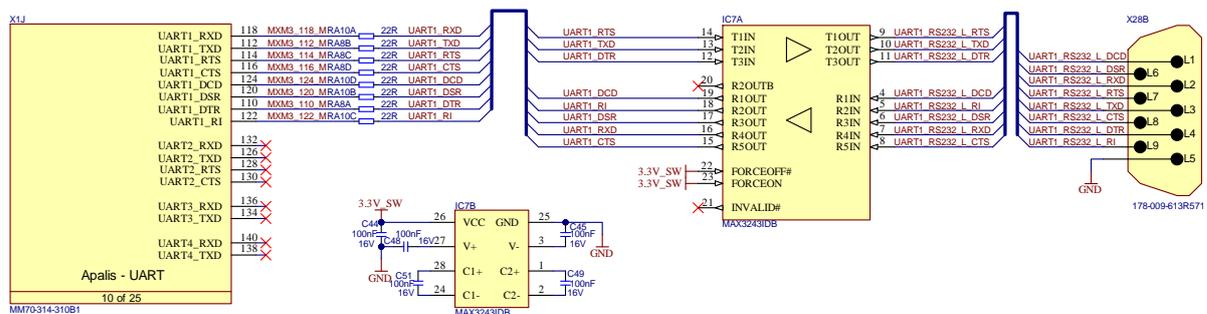
Figure 62: RS232 Reference Schematic
