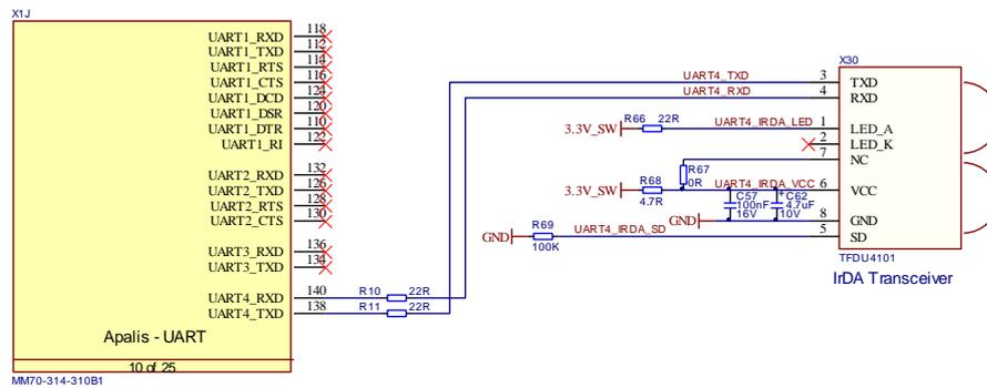
Figure 65: IrDA Reference Schematic
