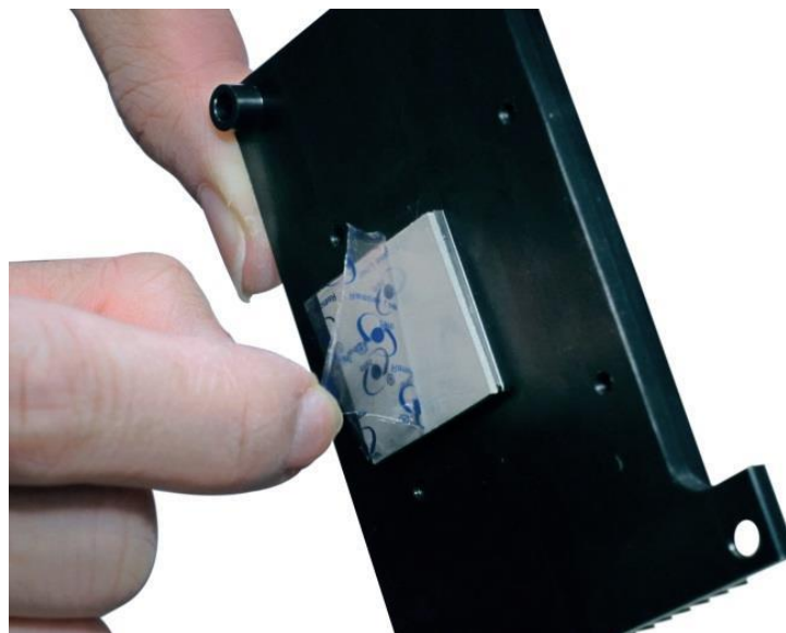
Figure 3: Remove plastic foil from the TIM
