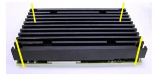
6. Use M2.5 screws to fix the heatsink together with module.
