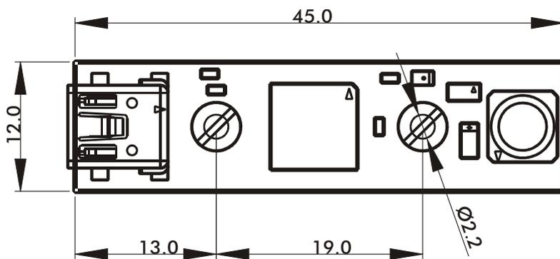
Figure 1: Mechanical dimensions of the Oak Tilt sensor
